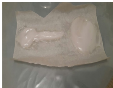
Picture 4 – Salt-soda bioplastic.
